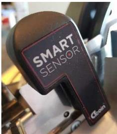
The SMARTconcept introduces a digital sensor, which uses a trio of EMS coils to sense and identify coins at high speed. Detected coin data is passed to the SMARTcontroller which handles ccTalk communication and coin module control. A connected computer retrieves the data from the controller for use in your application, either through ccTalk over standard serial communications, or using CTcoin's ccTalk API.
